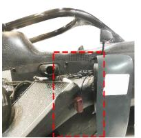
The mounting position of the transponder of a rechargeable or direct powered transponder is the same. The position must be identical on all cars competing in the championship. Fix the transponder vertically, at a maximum of 60cm (2ft) above the track. Make sure that the transponder has a clear view to the track with no metal or carbon fibre underneath. Maximum operating temperature should not exceed 122F/50°C.
